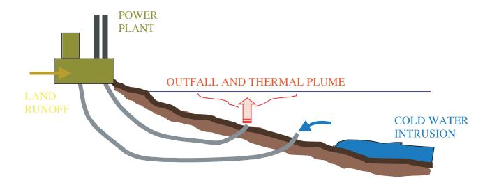
Figure 9-4. Schematic of power plant, showing thermal plume and cold-water intrusion.
