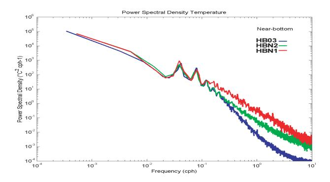
**Figure 9-5a.** Spectra of near-bottom temperature fluctuations on moorings HB03 (15 m, blue line), HBN2 (10 m, green line), and HBN1 (5 m, red line).
