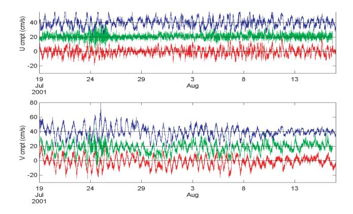
**Figure 9-6.** Near-bottom cross-shore velocities (upper panel) and alongshore velocities (lower panel) at HB03 (15 m, blue), HBN2 (10 m, red), and AES2 (6.5 m, green). Plots are offset 20 cm/s to separate lines–a zero line is shown for each trace. Note the decrease in both energy and coherence of cross-shore flows in the nearshore, in contrast to strong alongshore flows.
