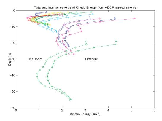
**Figure 9-7.** Energy density of cross-shore currents in each ADCP bin–across all frequencies (star and asterisk) and for internal wave frequencies only (open symbols). Data shown for moorings HB07 (green), HB06 (magenta), HB05 (blue), HB03 (cyan), HBN2 (yellow), AES3 (green), HBN3 (red), AES2 (magenta), and HBN1 (blue).
