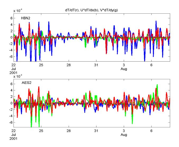
**Figure 9-9.** Summary of thermal balance calculations centered at HBN2 (10 m, top panel) and AES2 (6.5 m, bottom panel). The observed  $\partial tT$  is plotted in red, cross-shore advection u. $\partial xT$  in blue, and alongshore advection v. $\partial yT$  in green.
