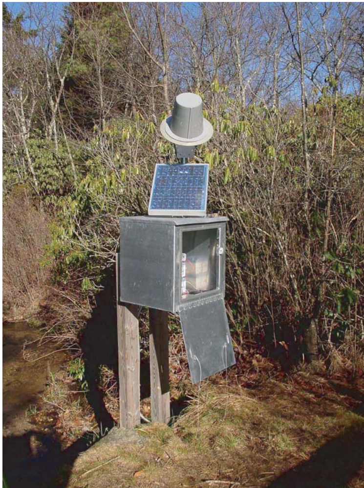
Figure 5. The U.S. Geological Survey gaging station that was built to monitor water levels in the stream flowing from the natural area in the center of the Mt. Pisgah campground.
