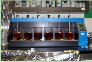
Experimental laboratory set-up employed to produce aggregate particles from dissolved organic matter present in Suwannee River water
