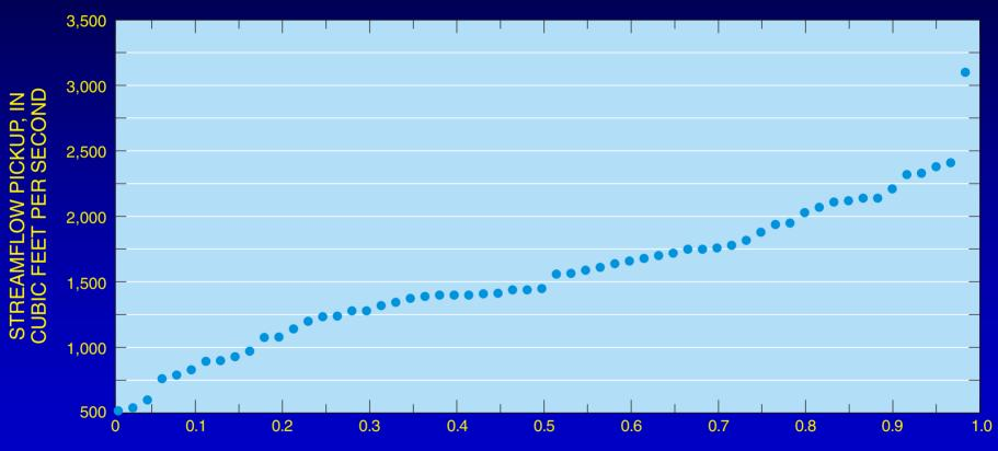
PROBABILITY OF EXCEEDING A GIVEN LEVEL OF STREAMFLOW PICKUP
