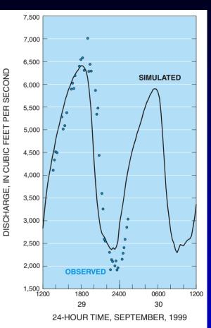
Simulated and observed flow in the Suwannee River upstream from the mouth of Manatee Springs Run during September 29-30, 1999.
