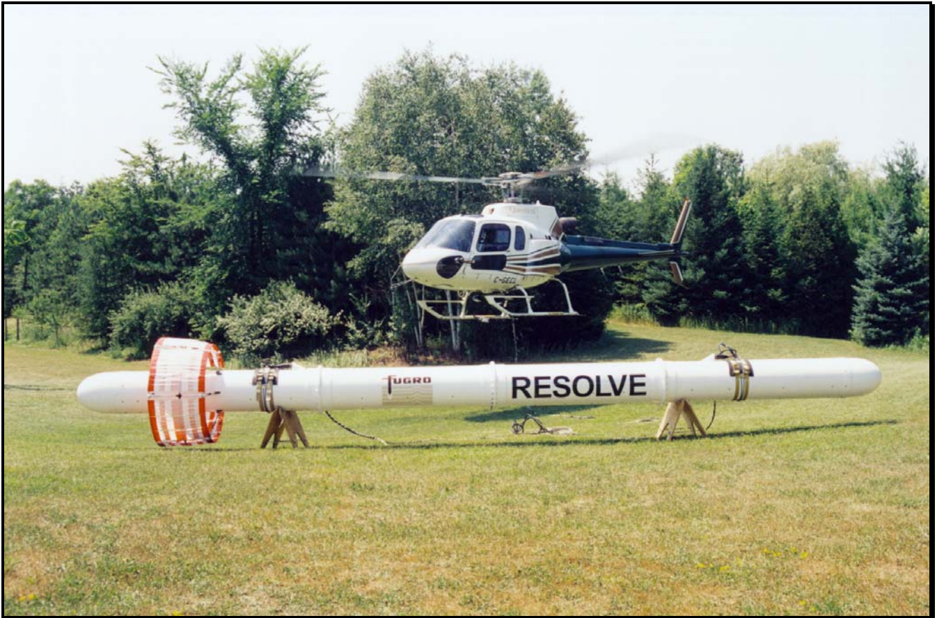
Figure 1: Fugro Airborne Surveys RESOLVE EM bird with AS350-B3
