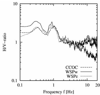
Figure 3. Comparison between arithmetic mean curves of spectral H/V-ratios on microtremors at the different recording sites.
