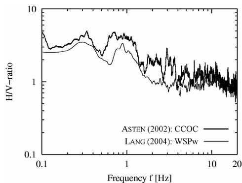
Figure 4. Spectral H/V-ratio on microtremors determined by LANG (2004; site WSPw) compared with that derived by ASTEN (2002; site CCOC).
