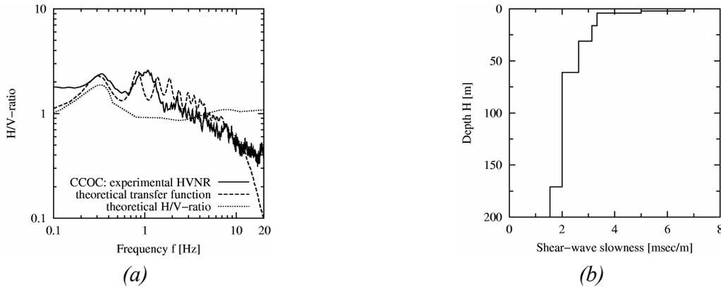
Figure 5. (a) Comparison between experimental transfer function (HVSR) and theoretical transfer functions of the derived subsoil profile, (b) corresponding shear-wave slowness model of the uppermost 200 m.
