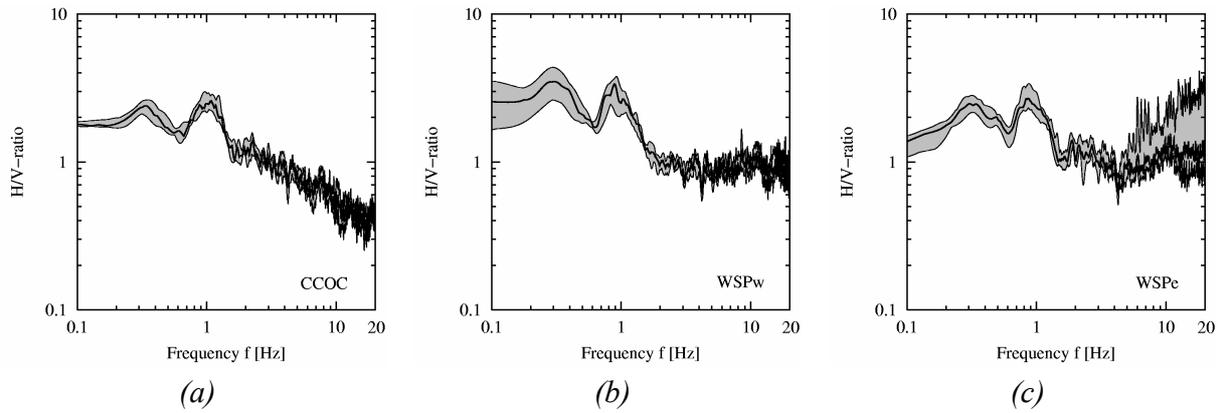
Figure 2. Spectral H/V-ratios on microtremor data recorded at the three different sites (bold line: arithmetic mean value, gray-shaded area: mean value  $\pm$  standard deviation).
