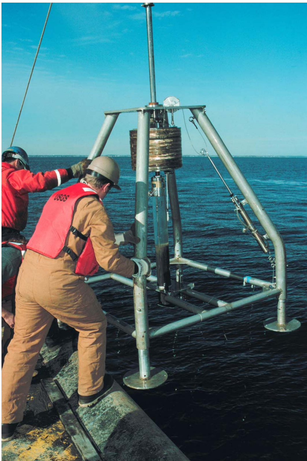
Figure 1.8. Sediment samples were collected with a hydraulically damped gravity corer, which collects sediment cores (10.7 cm internal diameter and up to 50 cm long) with minimal disturbance of material at the water-sediment interface (Bothner and others, 1997).
