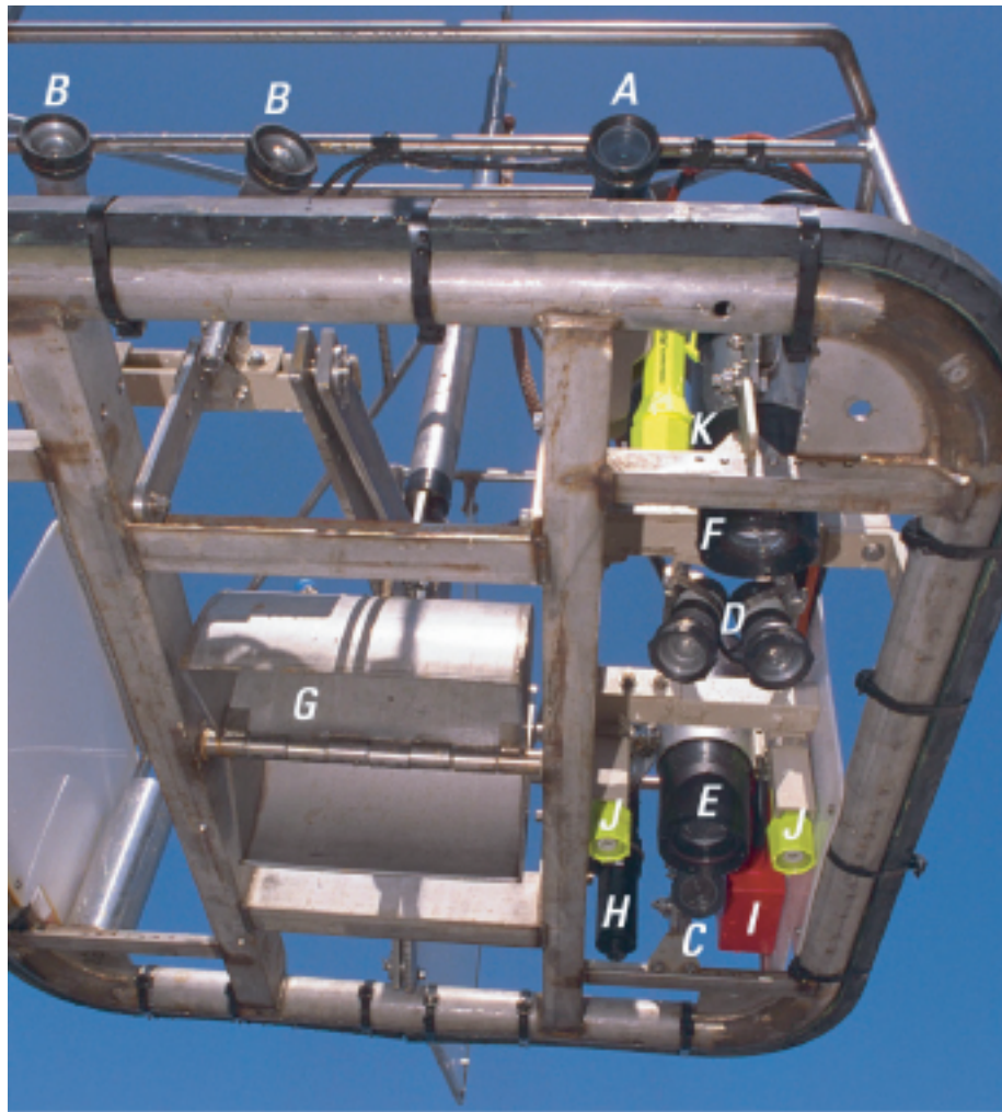
Figure 2.3. The USGS SeaBed Observation and Sampling System (SEABOSS) used to obtain still photographs, videos and obtain samples of the sea floor sediments. These observations are used to help interpret the backscatter intensity obtained in the multibeam surveys. The SEABOSS is lowered to within about a meter of the sea floor and obtains photographs and videos as the ship drifts over selected features. A single sample of the bottom sediments may be obtained during the photographic transect. Top: A view of the SEABOSS from below (with base plates removed). The instruments are as labeled: A, forward-looking video camera; B, lights for forward-looking video camera; C, downward-looking video camera; D, lights for downward-looking video camera; E, 35-millimeter still camera; F, strobe light for still camera; G, modified Van Veen grab sampler; H, depth sensor; I, junction box; J, parallel lasers for scale; K, angled laser for range. Right: SEABOSS on deck.
