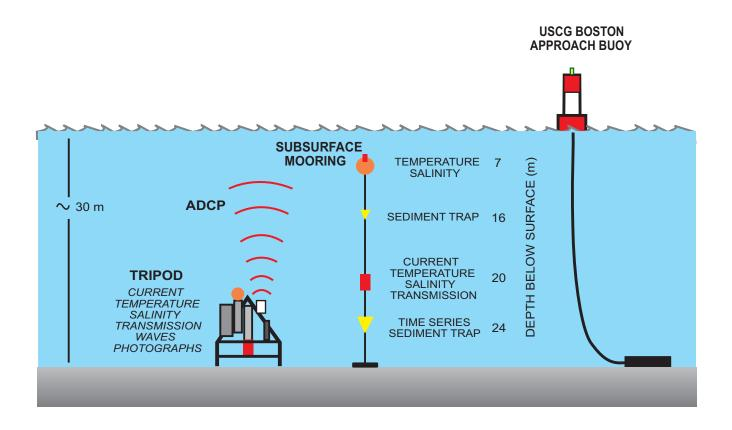
**Figure 3.2.** Schematic of moored instruments deployed at the long-term western Massachusetts Bay site LT-A from 1996 to 2005. During this period, instruments were deployed on a subsurface mooring and on a bottom tripod system. The acoustic Doppler current profiler (ADCP), mounted on the bottom tripod, obtains a profile of current throughout the water column in 2-meter bins.
