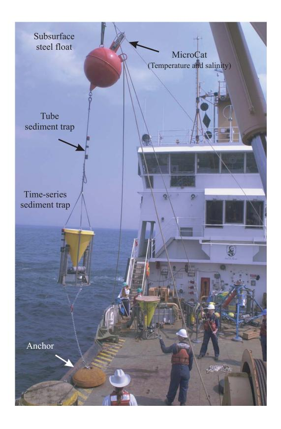
Figure 3.4. A subsurface mooring being deployed from the U.S. Coast Guard Cutter *Marcus Hannah* at LT-B.
