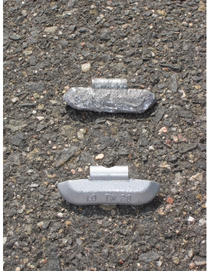
Figure 3. Clip-on 1-ounce lead-based wheel weights; comparison of a new weight and one abraded by traffic (photo source: Donald I. Bleiwas).
