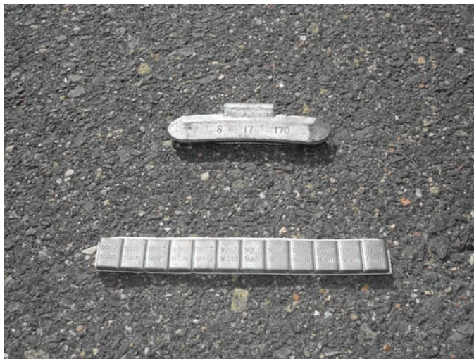
Figure 1. Six-ounce clip-on and 6-ounce adhesive-backed lead weights for use on larger vehicles, such as buses and trucks (photo source: Donald I. Bleiwas).
