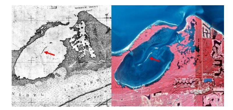
Figure 29. The Tarpon Bay Keys (red arrows), Florida, as depicted on topographic sheet T-693 from 1859 (left) and in a 1999 false color infra-red aerial photograph. The two images are not to equal scales.
