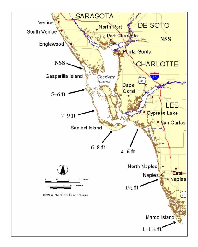
Figure 8. Visually estimated open coastal high water levels during Hurricane Charley (based on unsurveyed estimates subject to change and corrections) August 24, 2004. Data and Figure provided to USGS by the Coastal High Water Study Team under the Federal Emergency Management Agency (FEMA).
