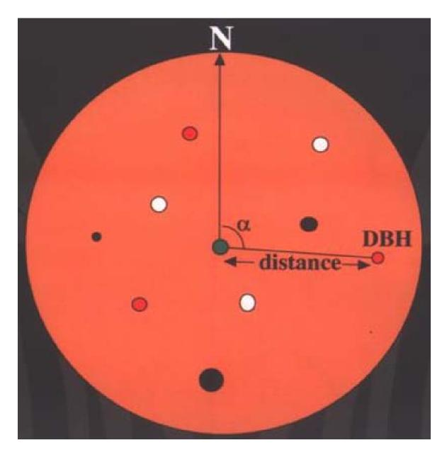
Figure 44. This figure shows a schematic view of the plot layout (orange circle) used by the USGS for mangrove vegetation studies in coastal Everglades, Florida. From the permanent center stake (green dot), the distance and bearing (α) from North (N) to each stem is recorded as well as the diameter breast height (DBH) and species.
