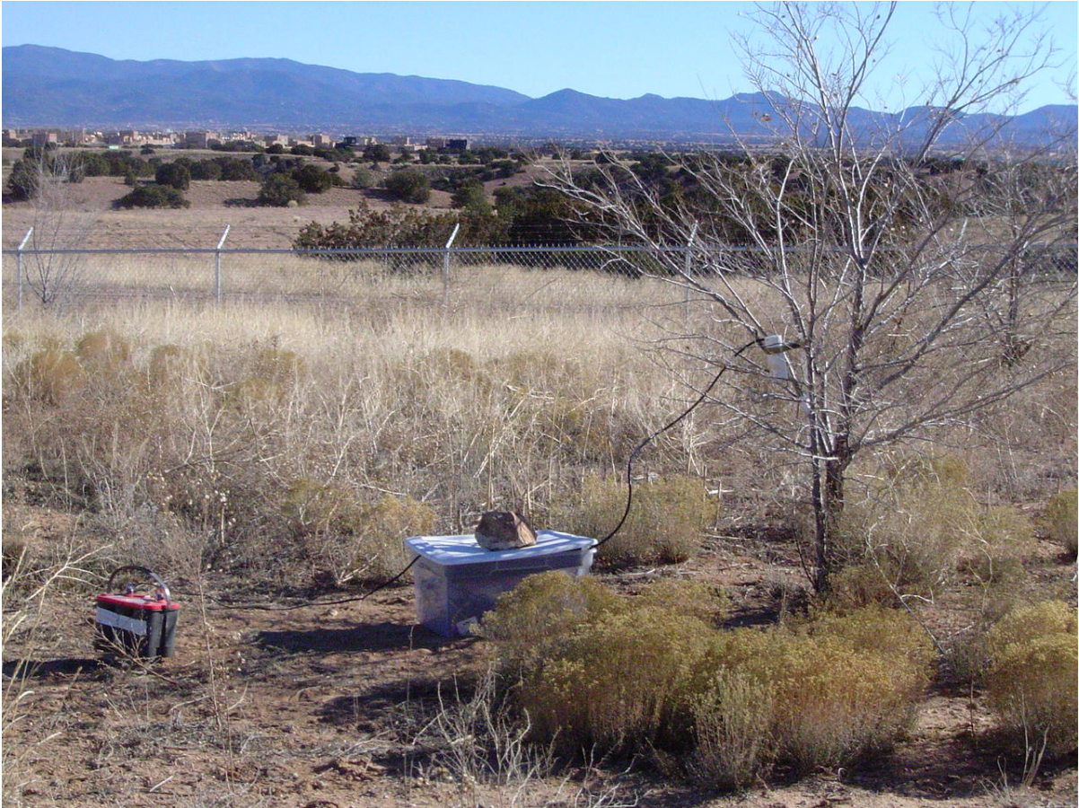
Figure 2-3A. The magnetic base station with GPS RF-link in Santa Fe Airport
