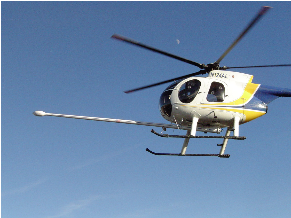
Figure 2.4 Stinger mounted Helicopter magnetometer survey system
