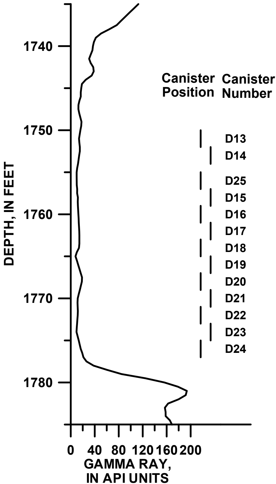
Core Hole 11B. Gamma Ray, canister position, and canister label for the Barrett Resources Corporation CARU State 22-16-5074W core hole showing the Werner coal bed.
