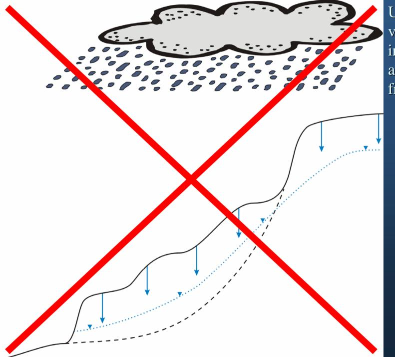
Uniform vertical infiltration of a saturation front
