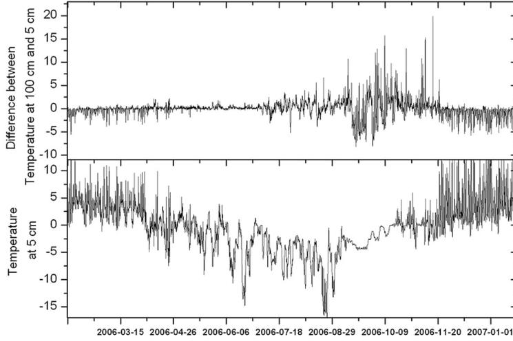
**Figure 2.** Data from the thermal snow layer probe sited close to Incinerator borehole during 2006. Top: The temperature difference between the readings at 100 cm and 5 cm. Bottom: the annual temperature profile measured at 5 cm above ground at the Incinerator site.
