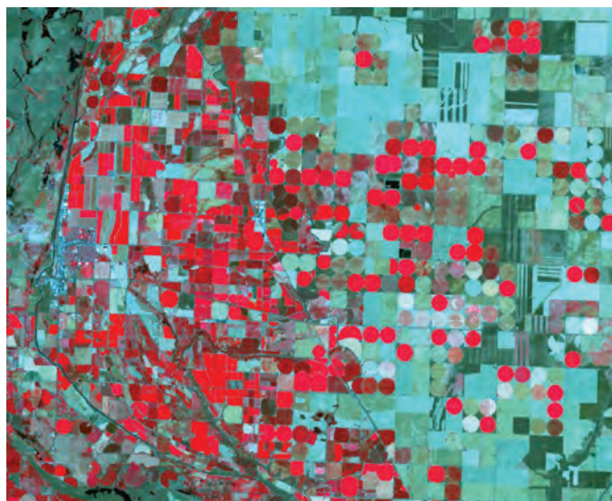
Figure 2. Enhanced Thematic Mapper Plus image subscene over EL68D Wasteway Watershed, July 12, 2001. Bands 4, 3, and 2 are shown in red, green, and blue, respectively.
