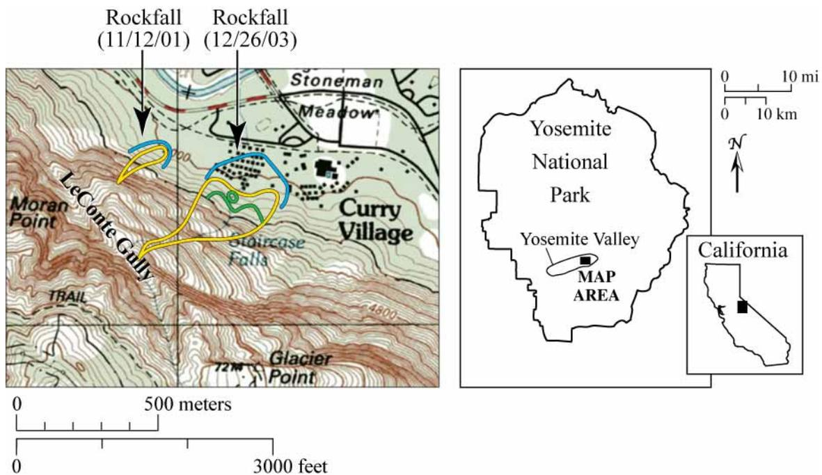
**Figure 1.** Topographic map of Glacier Point-Curry Village in Yosemite Valley, California, with two rockfalls from Staircase Falls into Curry Village. Yellow lines show the initial release, travel track, and continuous rock debris deposit region. The green line depicts where trees were knocked down, and the blue lines show the limit of flyrock.
