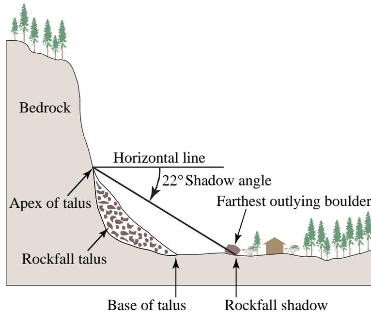
**Figure 4.** Sketch of rockfall talus at base of slope and outlying boulders illustrating the limit of the rockfall shadow angle (Wiczorek and others, 1999).
