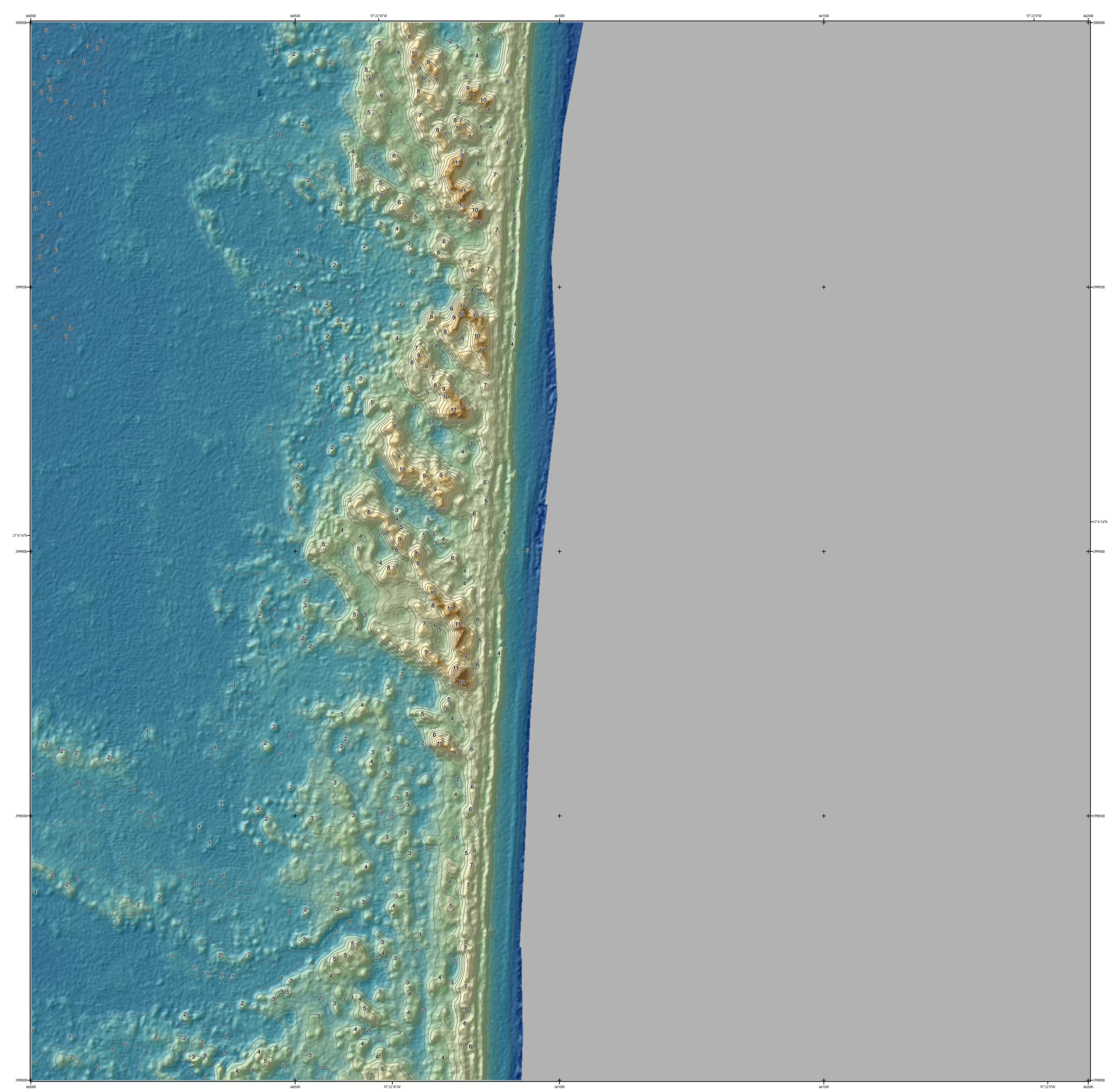
Universal Transverse Mercator. 1983 North American Datum-Zone 14 North Topography mapped using NASA Experimental Advanced Airborne Research Lidar (EAARL) September/October 2005 This map is not intended for use in navigation.
