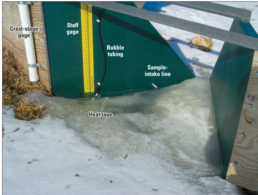
Figure 8. Ice was removed from H flumes before runoff events. Here, icemelt near the bubble line and sample-intake line due to the heat tape can be seen.
