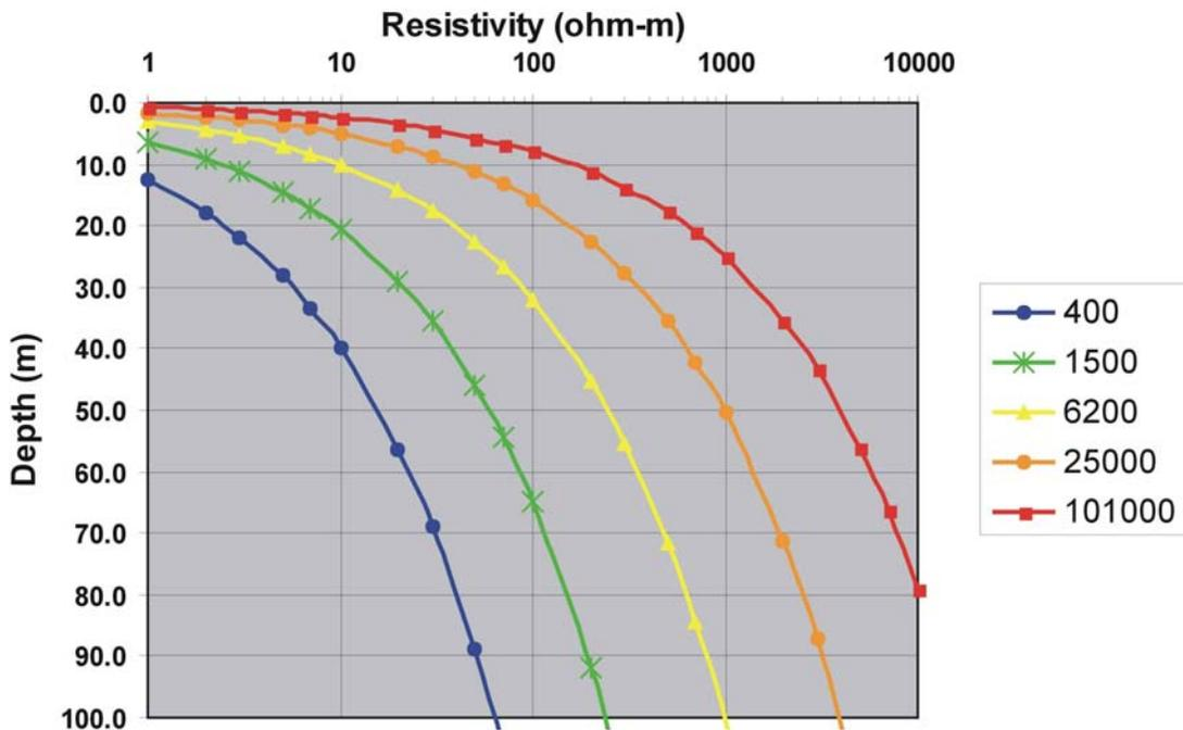
**Figure 4.** Estimated depth of penetration or imaging as a function of frequency and earth resistivity for the RESOLVE© system (Hodges, Fugro Airborne, 2004, written commun.).
