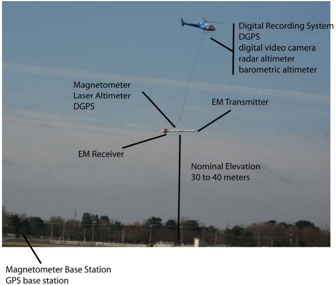
**Figure 3.** Helicopter-borne Resolve geophysical system used in the Nebraska survey flying near Fremont, NE: Electromagnetic, magnetic, DGPS, and laser altimeter sensors are housed in a “bird”, a cigar-shaped 9-m-long tube, which is kept at about 30–40 m above ground level. The digital data recording system, additional altimeters, and navigation systems are installed in the helicopter. The base station records the time-varying, diurnal, total magnetic field variations.
