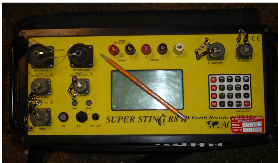
Figure C-9. The DC resistivity SuperSting R8 console.
