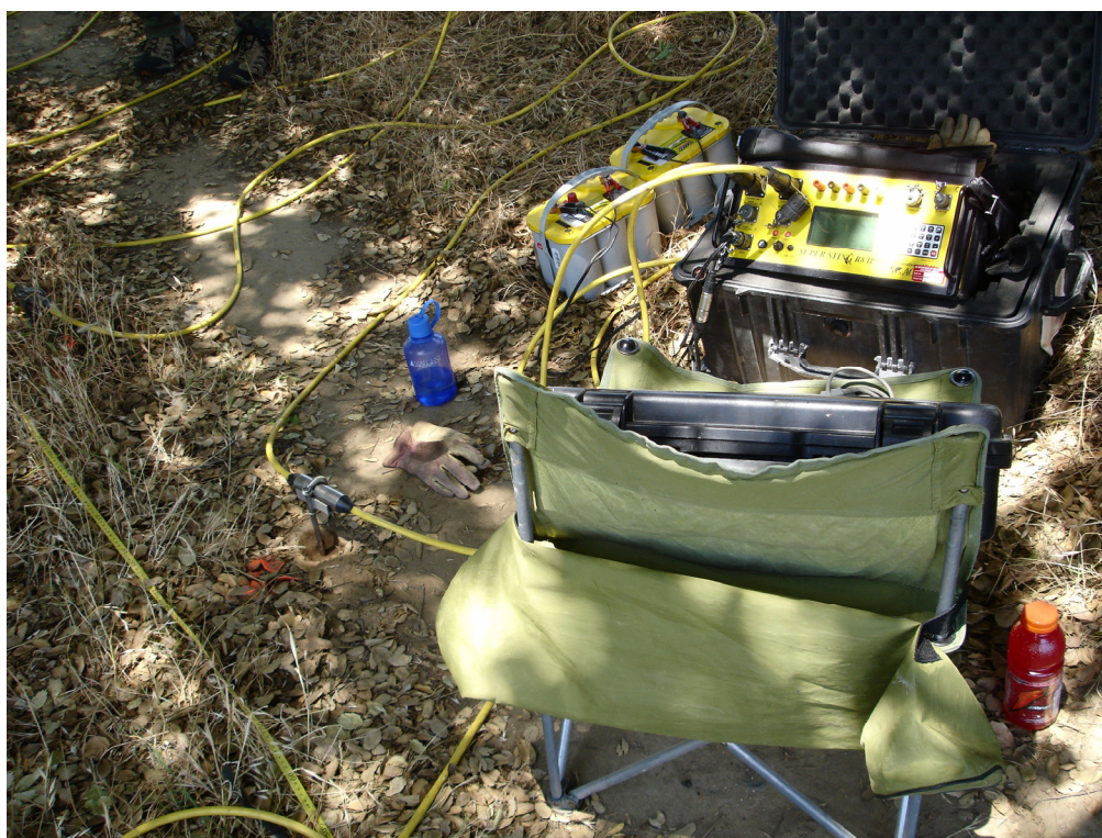
Figure C-10. The SuperSting deployed along the horse trail.
