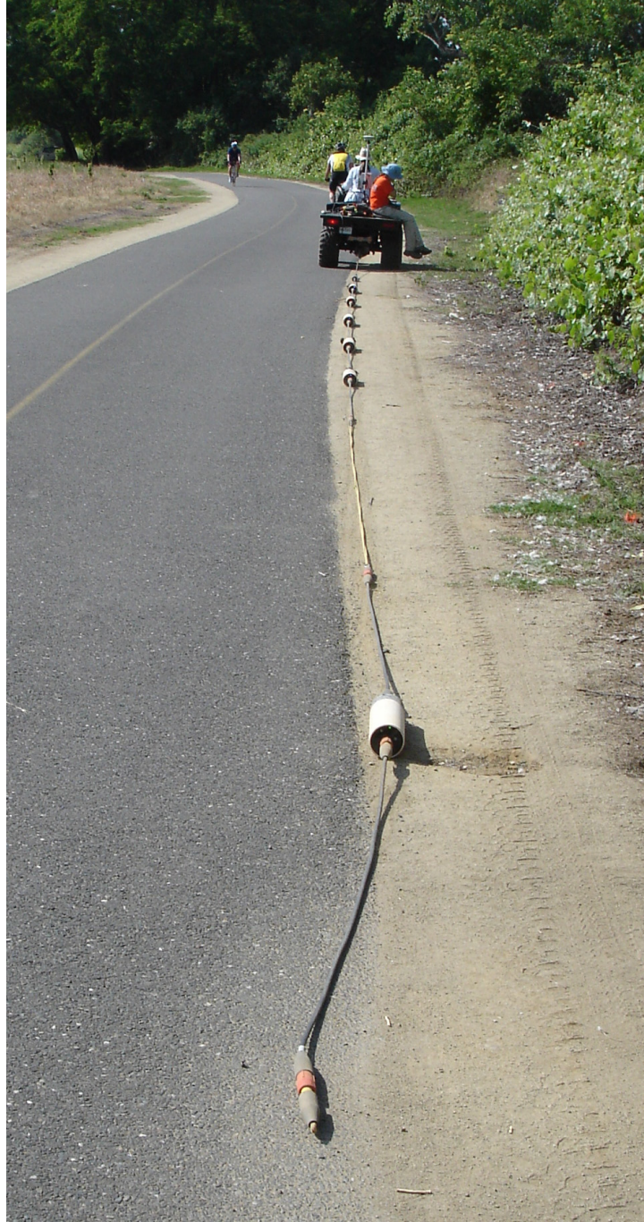
Figure C-1. The OhmMapper deployed along the bike trail.
