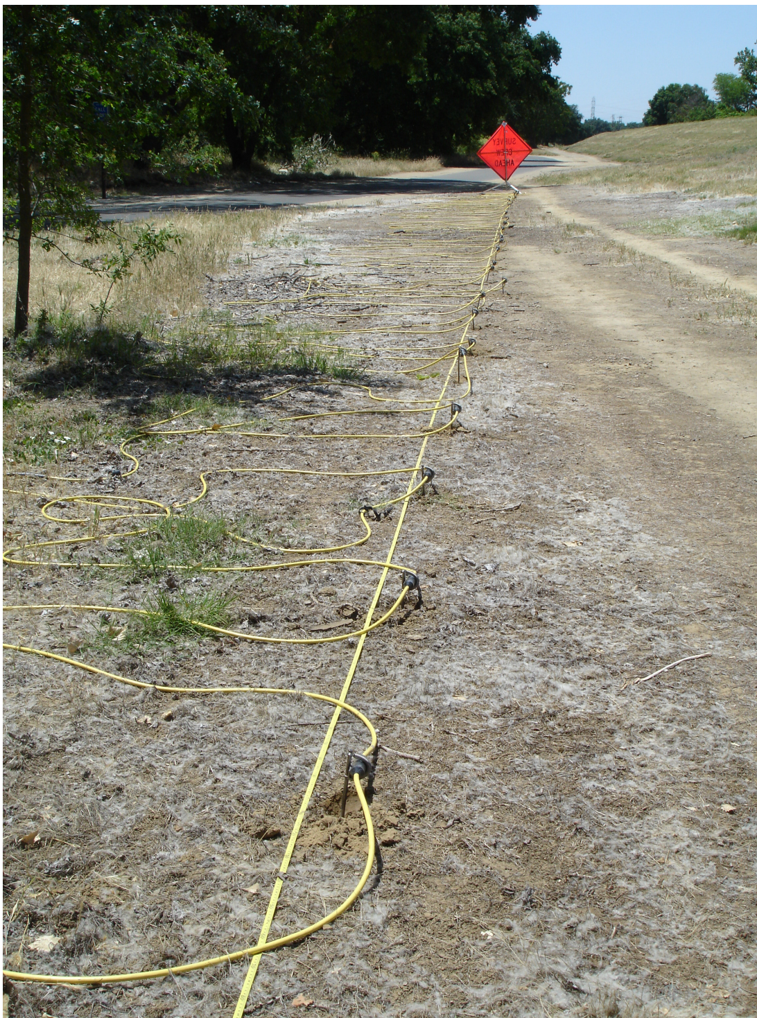
Figure C-8. The DC resistivity cable deployed along the bike trail.
