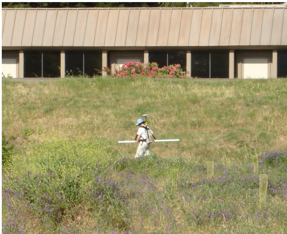
Figure C-6. The GEM-2 deployed along the bike trail.
