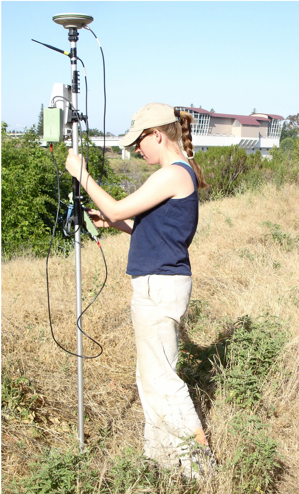
Figure C-11. Recording the locations of specific survey features.
