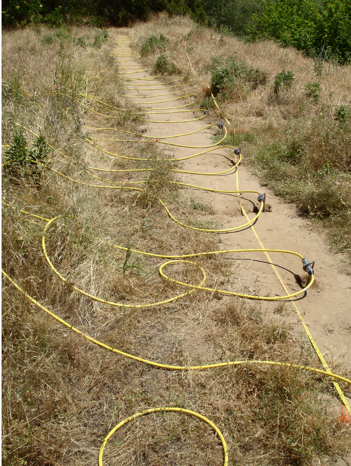
Figure C-7. The DC resistivity cable deployed along the horse trail.
