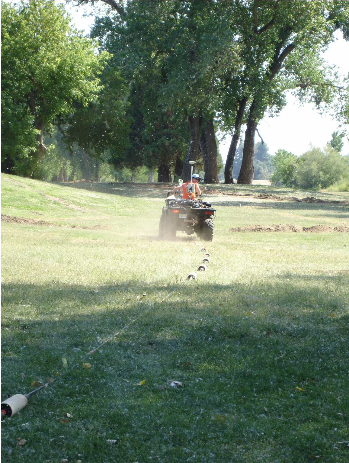
Figure C-2. The OhmMapper deployed the Campus Commons Golf Course.
