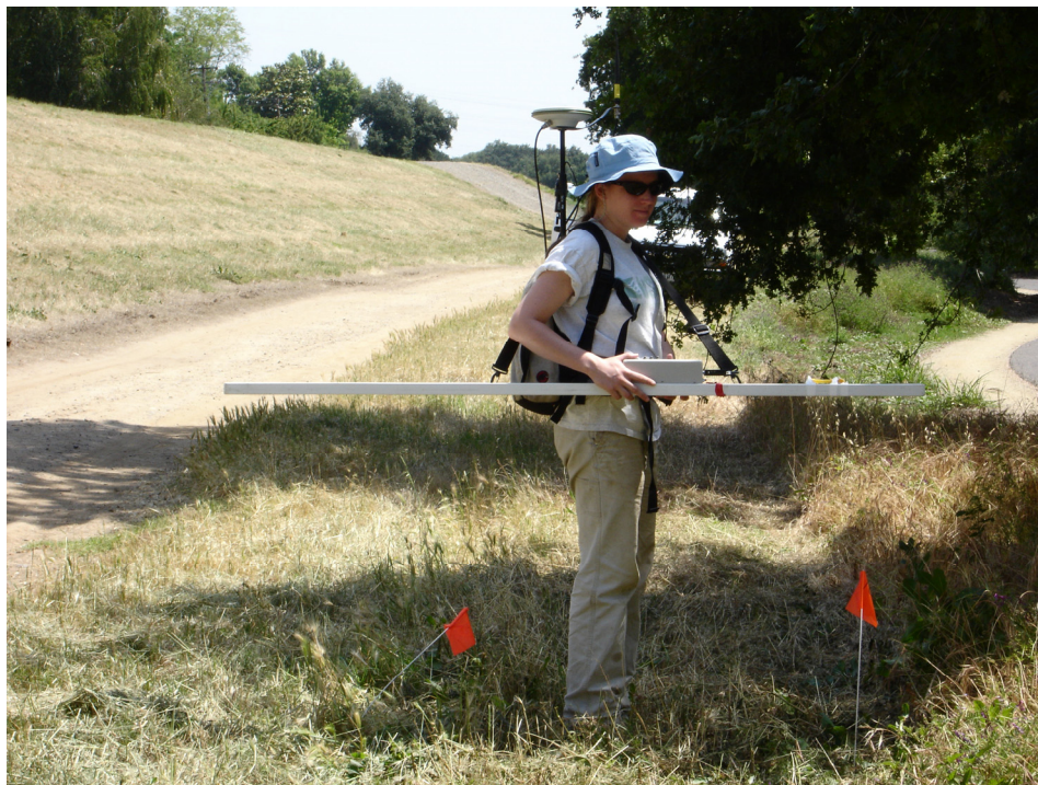
Figure C-5. The GEM-2 deployed along the levee toe road.
