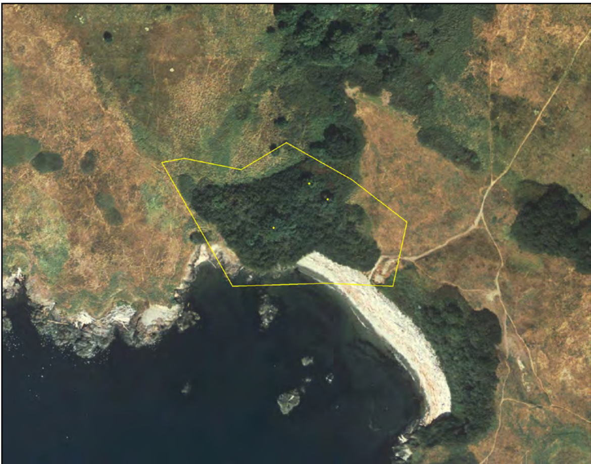
Figure 4. American Camp orthoimage, 1997. Dark green area surrounded by the yellow polygon was originally misclassified as forest as a result of the longer shadows cast at the time of year the imagery was flown.
