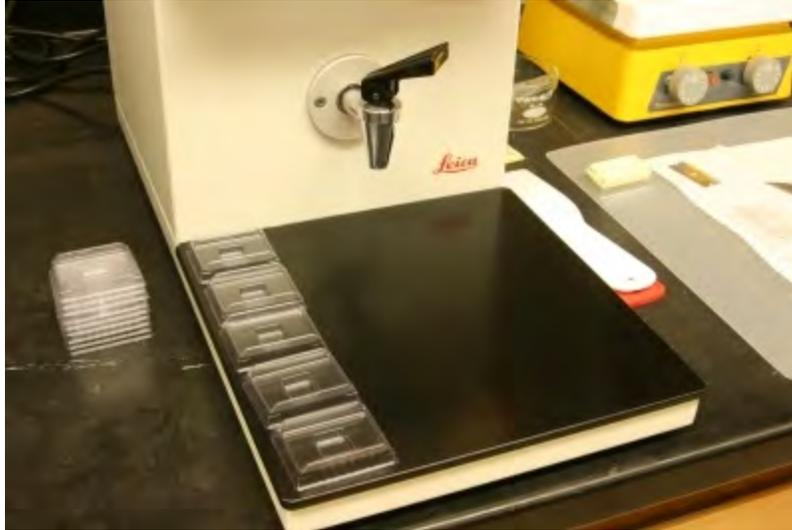
**Figure 6.** Molds pre-warming on hot plate.
