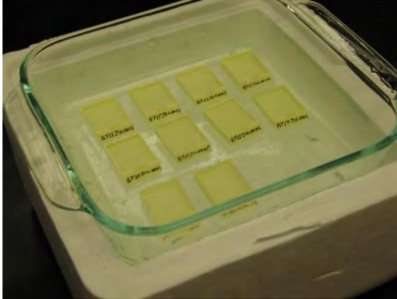
**Figure 9.** Paraffin blocks cooling in the cold tray, prior to facing or sectioning.
