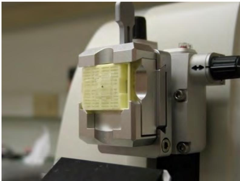
**Figure 10.** Paraffin-block clamped in microtome chuck.
