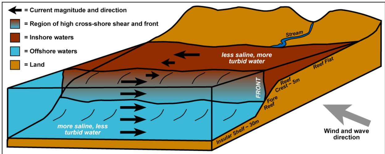
**FIGURE 3.** Schematic displaying the nature of flow and water column properties resulting in a front along West Maui. Higher turbidity and submarine groundwater discharge or freshwater runoff is typically found close to shore. Along the relatively straight sections of coast, net wave- and wind-driven flow close to shore is downwind. Flow farther offshore is upwind, causing zones of high cross-shore horizontal velocity shear and often fronts.
