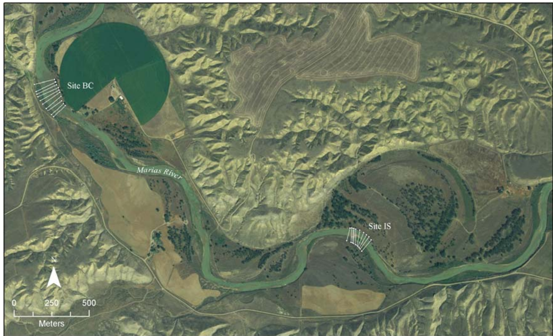
Figure 5. Aerial imagery of study region on lower Marias River from 2005. Head pins of cross sections at Sites IS and BC are depicted as solid circles. Grid lines are Universal Transverse Mercator (UTM, Zone 12) projection of latitude and longitude referenced to NAD 83(99) horizontal datum. Note contrast between width of cross sections containing the post-dam flood plain and the width of the zone containing mature cottonwood trees and relict channel locations. Imagery is from National Agriculture Imagery Program (2005).
