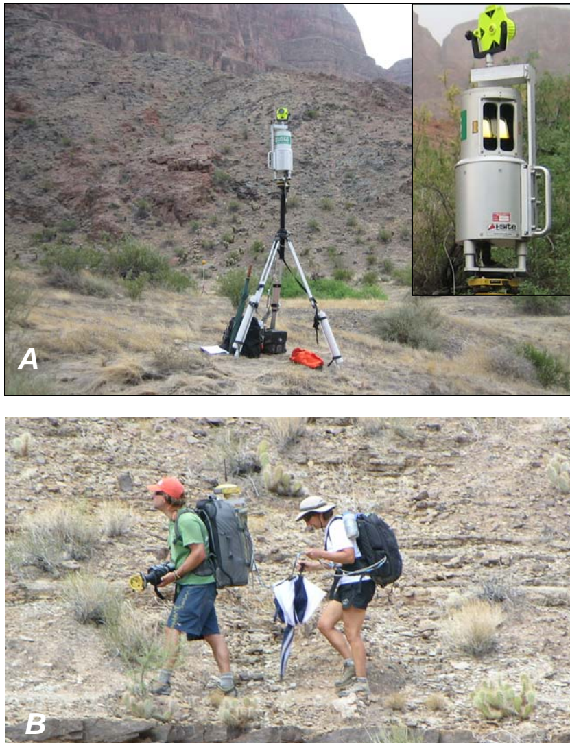
Figure 5. A , Terrestrial light detection and ranging (LIDAR) data collection in Grand Canyon, Ariz. Extendable tripod allows a larger area of data collection and less oblique laser returns from flat ground. Inset shows laser pulse and return windows and survey prism used to georeference the instrument location. B , Transporting the system requires two people in most cases, the first to carry the laser and tripod and the second to carry the data acquisition unit (laptop computer) and laser batteries.
