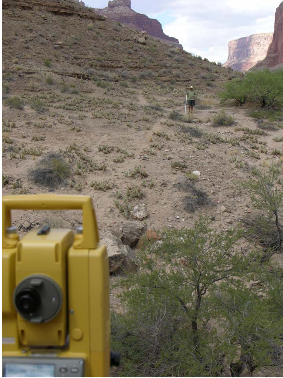
Figure 11. Conventional total station data collection showing use of survey rod and prism in a gully system. Communication between the surveyor at the total station and the personnel in the gullies is achieved through a combination of voice, arm signals, or handheld two-way radios.
