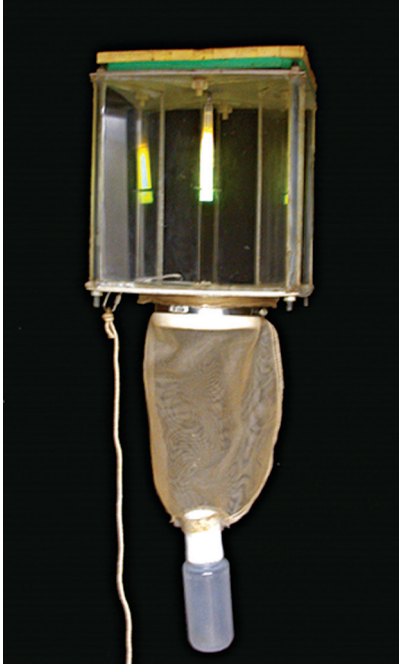
Figure 3. Light trap used to collect age-0 fishes in the Apalachicola River and floodplain. Luminescent chemical sticks were used in 2002-2004; a battery-operated white light was used in 2006-2007.
