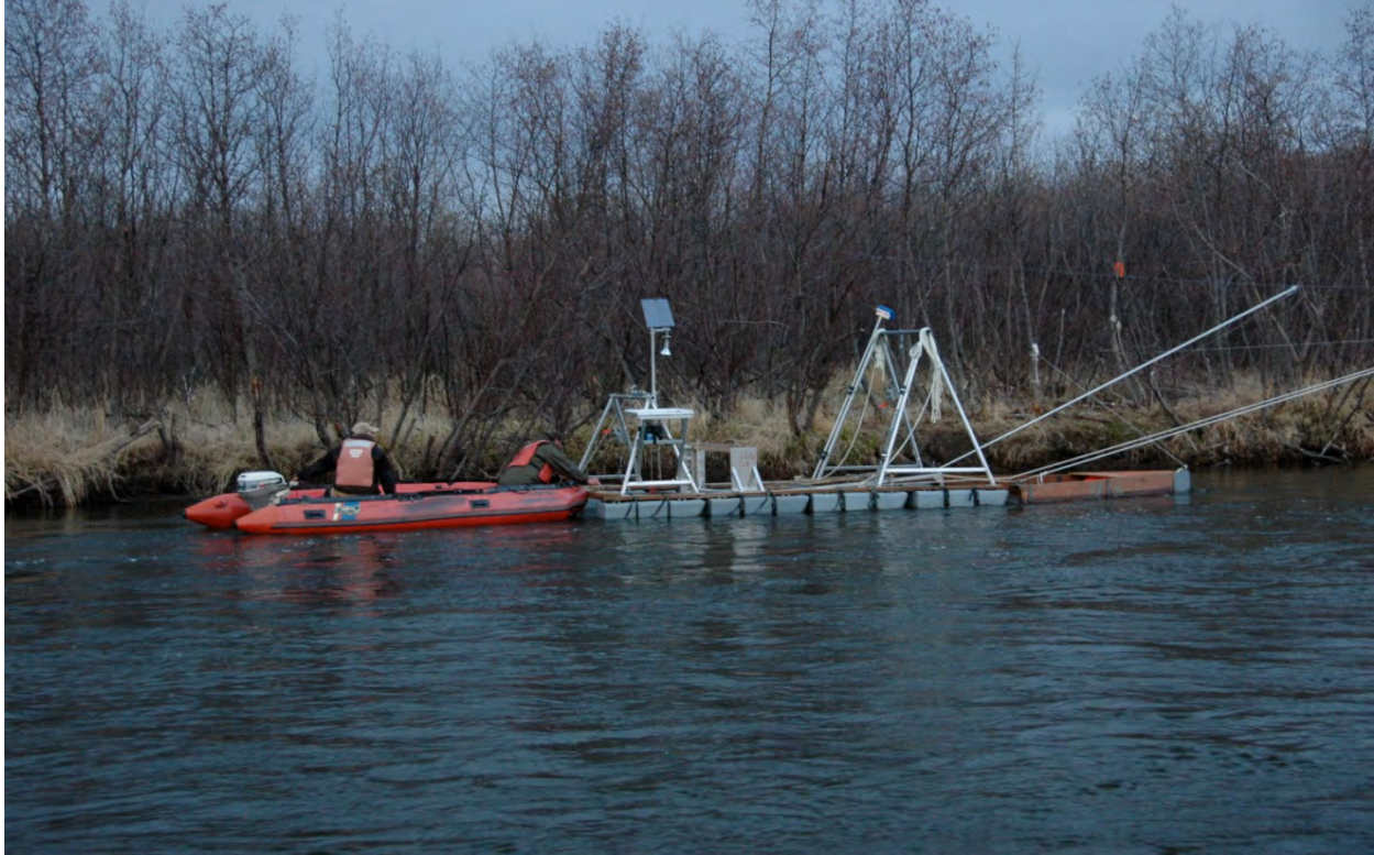
Figure 4. Inclined plane trap with ice-breaker bow attached, Kwethluk River, Alaska.
