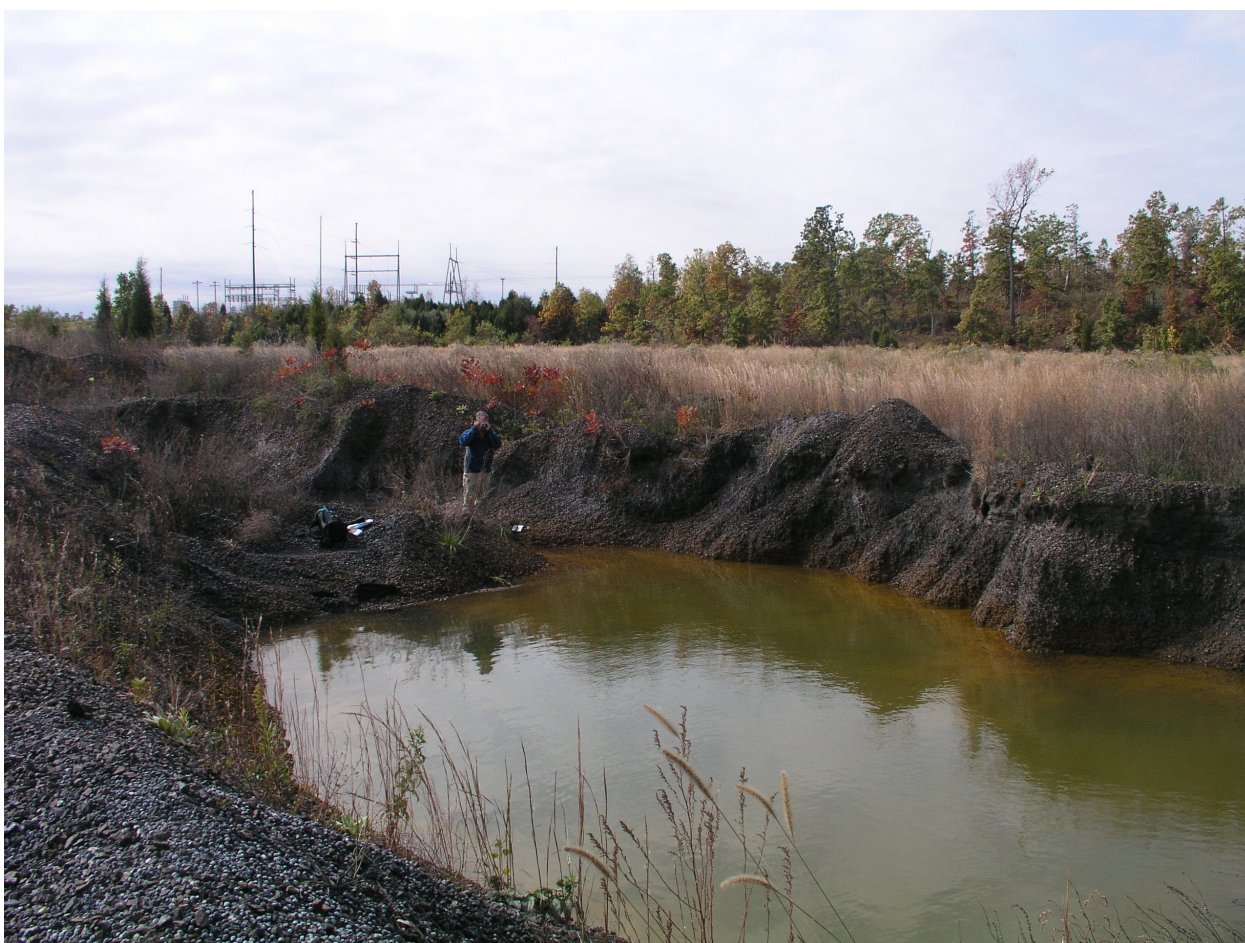
Figure 2. Small pool on tailings pile, Pea Ridge Mine, site of water sample 08MO01. Note orange alteration above and below water level and well-developed grasslands on reclaimed tailings in background. (P.L. Verplanck standing on the bank).
