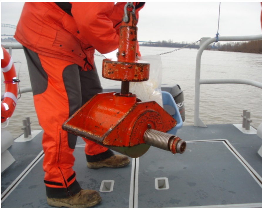
Preparing to collect bed-sediment sample from the Shipek grab sampler (Photograph by Daniel M. Wagner, U.S. Geological Survey).
