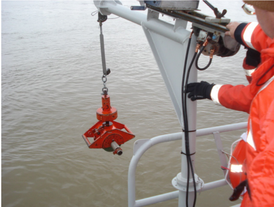
Retrieval of the Shipek grab sampler with bed-sediment sample (Photograph by Robert A. Blanchard, U.S. Geological Survey).
