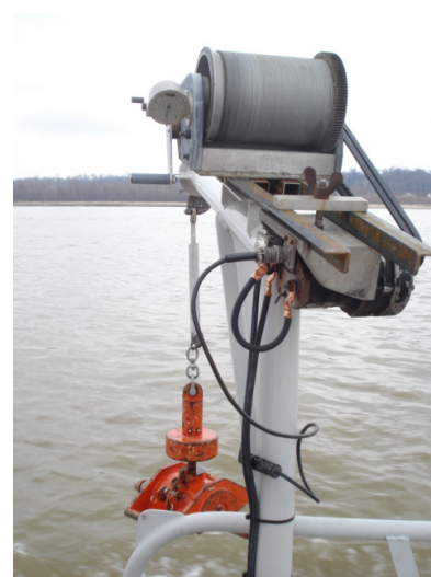
Deployment of the Shipek grab sampler for collection of bed sediment (Photograph by Robert A. Blanchard, U.S. Geological Survey).
