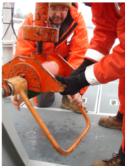
Preparing the Shipek grab sampler for collection of bed sediment (Photograph by Robert A. Blanchard, U.S. Geological Survey).
