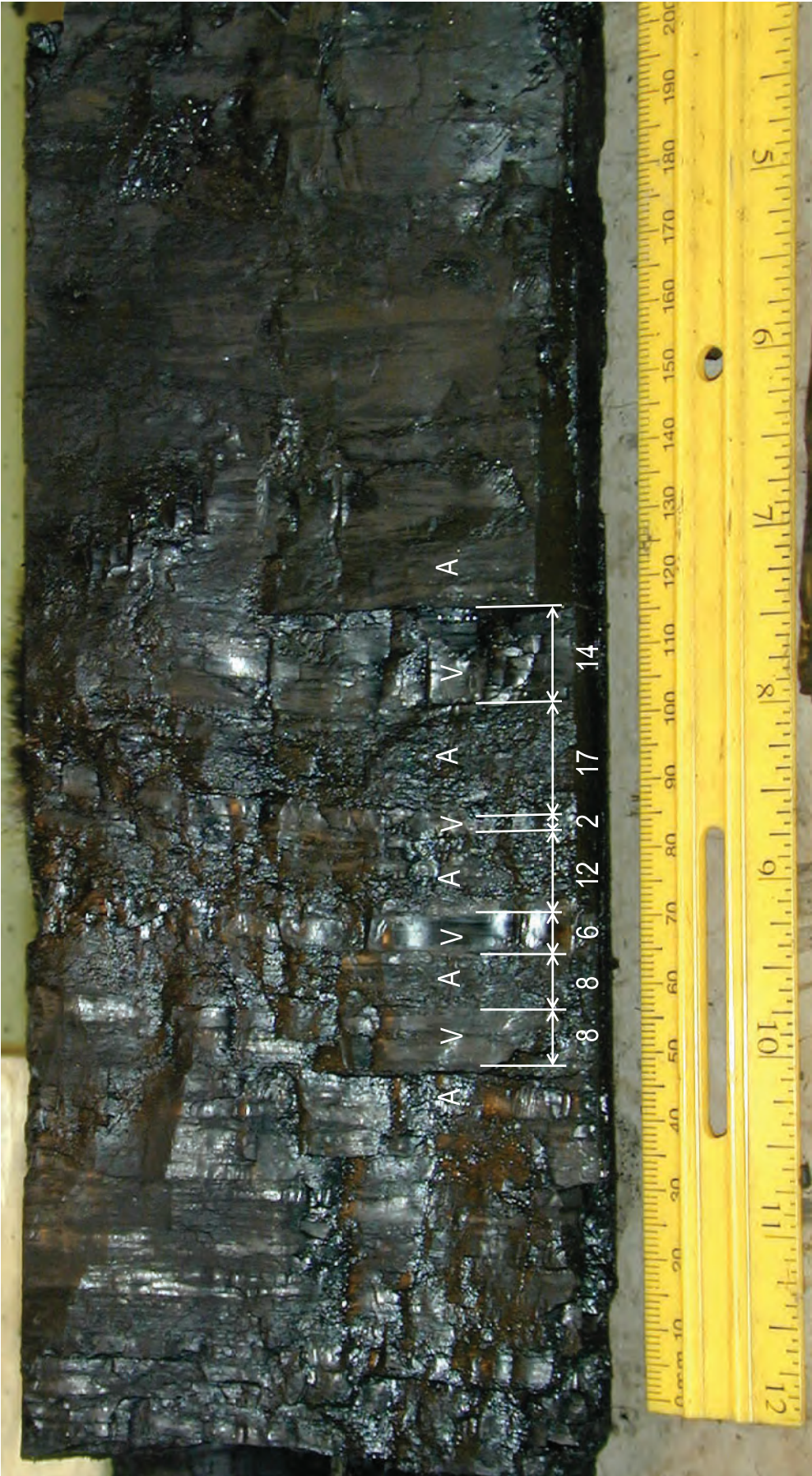
Figure 5. Photograph of canister coal sample split open for examination of megascopic lithologic features. Notice alternating vitrain (V, shiny) and attritus (A, dull) bands. Thicknesses of vitrain and attritus bands were measured in millimeters with the ruler.
