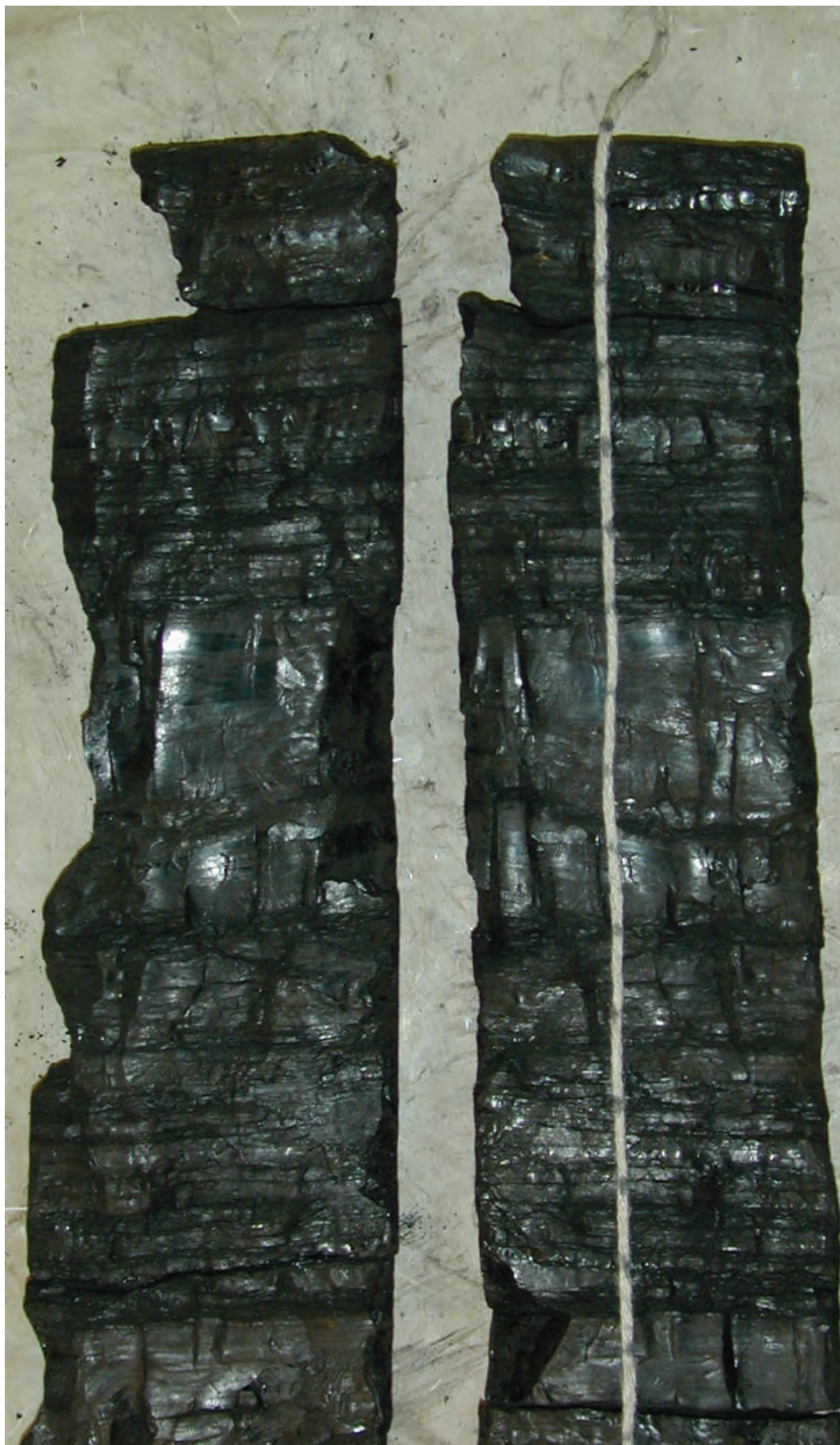
Figure 7. Photograph of canister coal sample with a string that is marked at 2-cm intervals and was used for the point-counting procedure. At this location, 11 bands of vitrain with a total thickness of 218 mm were recorded, resulting in an average vitrain band thickness of 19.8 mm (218/11). Assuming an equal number of attrital and vitrain bands, an average attrital thickness of 33.8 mm was calculated ((590-218)/11 , where 590 mm is the total canister thickness). Using these values for average vitrain and attrital band thicknesses a lithotype code of 3 (medium to coarsely laminated attritus and vitrain) was determined from the lithotype matrix (fig. 6).
