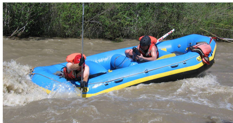
Rio Blanco River in Colorado. Field survey and velocity measurement from a raft at bankfull flow. USGS photo by Chris Holmquist-Johnson.
