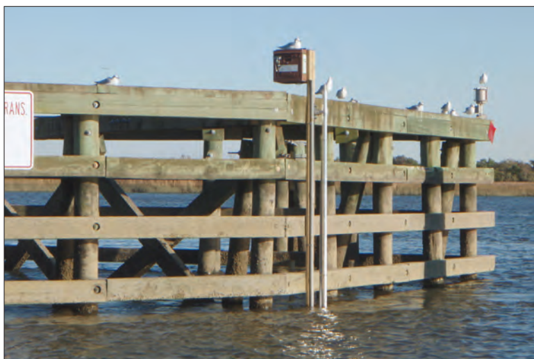
(Above) Figure 5. View of the instrumentation mount and housing at the Front River continuous index-velocity site, Lower Savannah River estuary, coastal South Carolina and Georgia (320954081092100; see fig. 2 for location).
