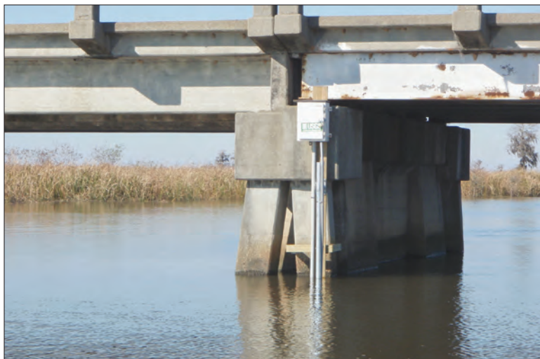
(Above) Figure 3. View of the instrumentation mount and housing at the Little Back River continuous index-velocity site, Lower Savannah River estuary, coastal South Carolina and Georgia (320957081074800; see fig. 2 for location).
