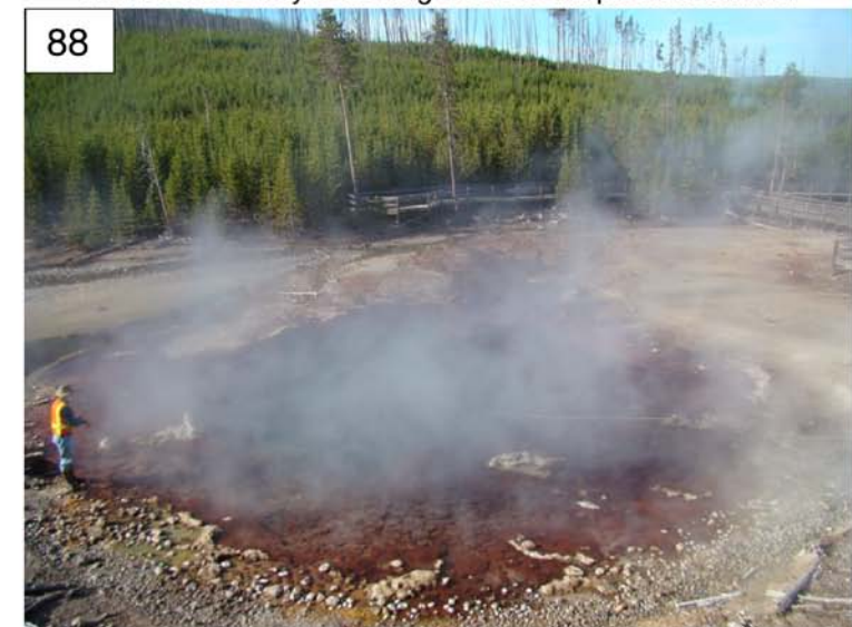
Kirk Nordstrom positioning the sample intake tubing at 08WA126, Echinus Geyser
