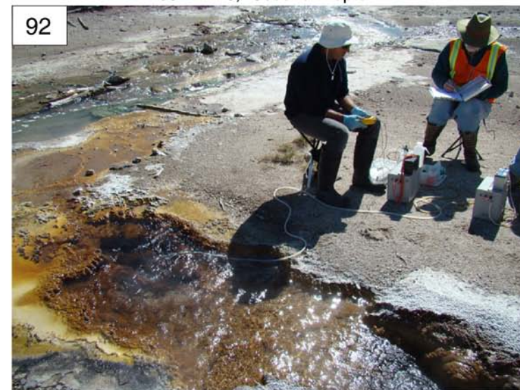
Nuno Durães and Kirk Nordstrom measuring pH at 08WA130, Perpetual Spouter
