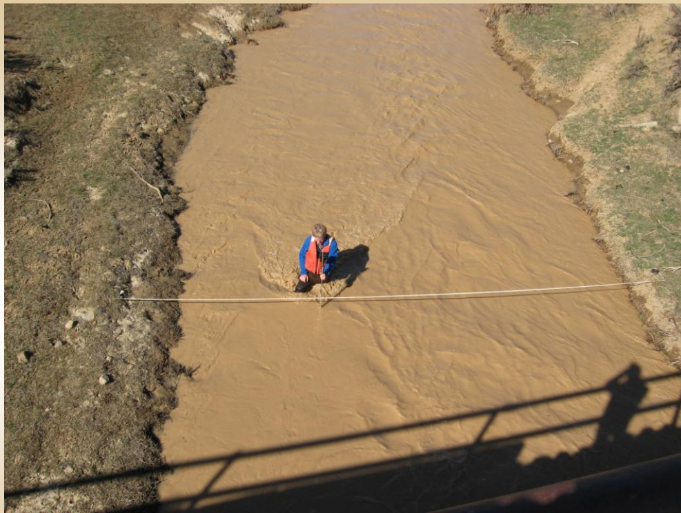
Wil Sadler measuring streamflow at USGS 09258980 Muddy Creek stream gage and water-quality monitoring site below Young Draw near Baggs, Wyoming, April 2008. Cooperator: U.S. Bureau of Land Management.
