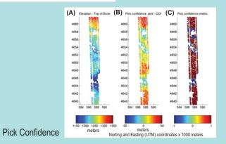
Plot of the picked HEM survey block collected in the North Platte Valley showing from left to right (A) Color plot of the interpreted pick elevation in meters
