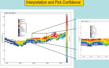
A selected 2-D resistivity image section (with zoom) showing location of test holes with lithology (vertical color bars), interpreted bedrock (black dots), and pre-HEM bedrock contour (gray line). The HEM data provided a better solution to the bedrock surface than just the test holes alone. All of the test hole data are correctly fitted with the HEM depth images. A set B and no transpanrency has been used.
