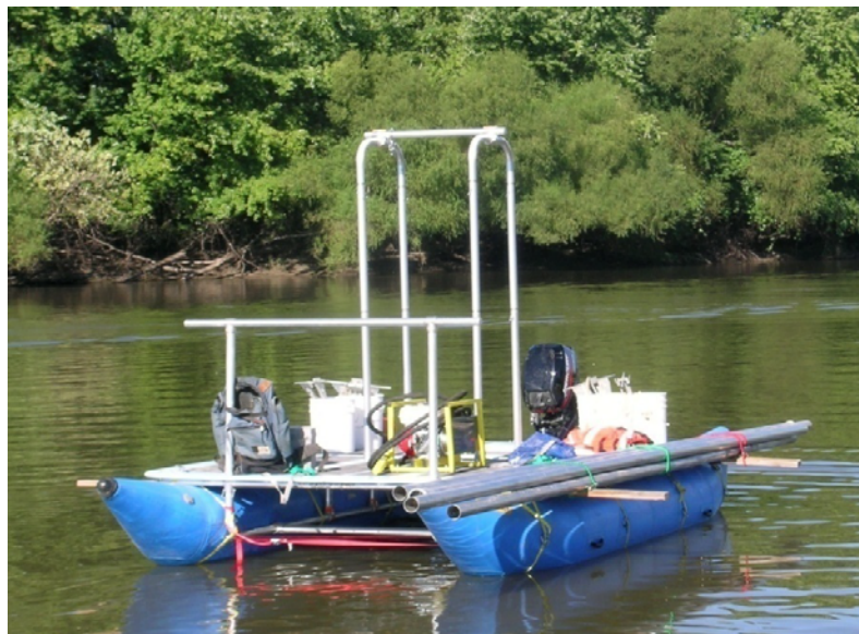
Figure 2. Pontoon boat coring platform. Aluminum tower is for attaching hand-operated winch to hoist core barrel.
