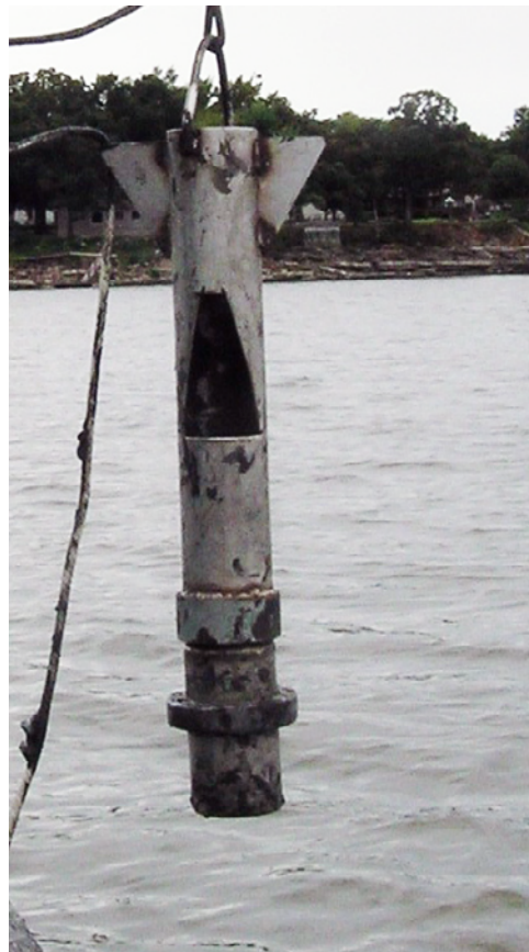
Figure 4. Simple gravity corer used to collect reservoir bottom-sediment samples.
