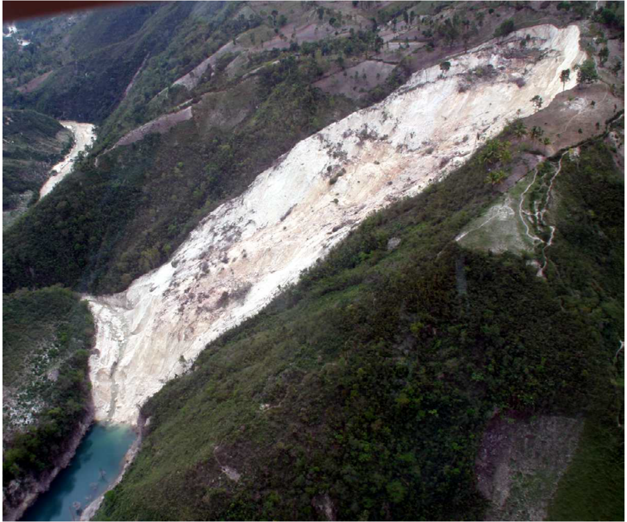
Figure 8. Landslide dam 15 kilometers northwest of Jacmel. The dam has breached, and the small amount of water impounded upstream should pose no future hazard. The landslide is about 150 meters wide.
