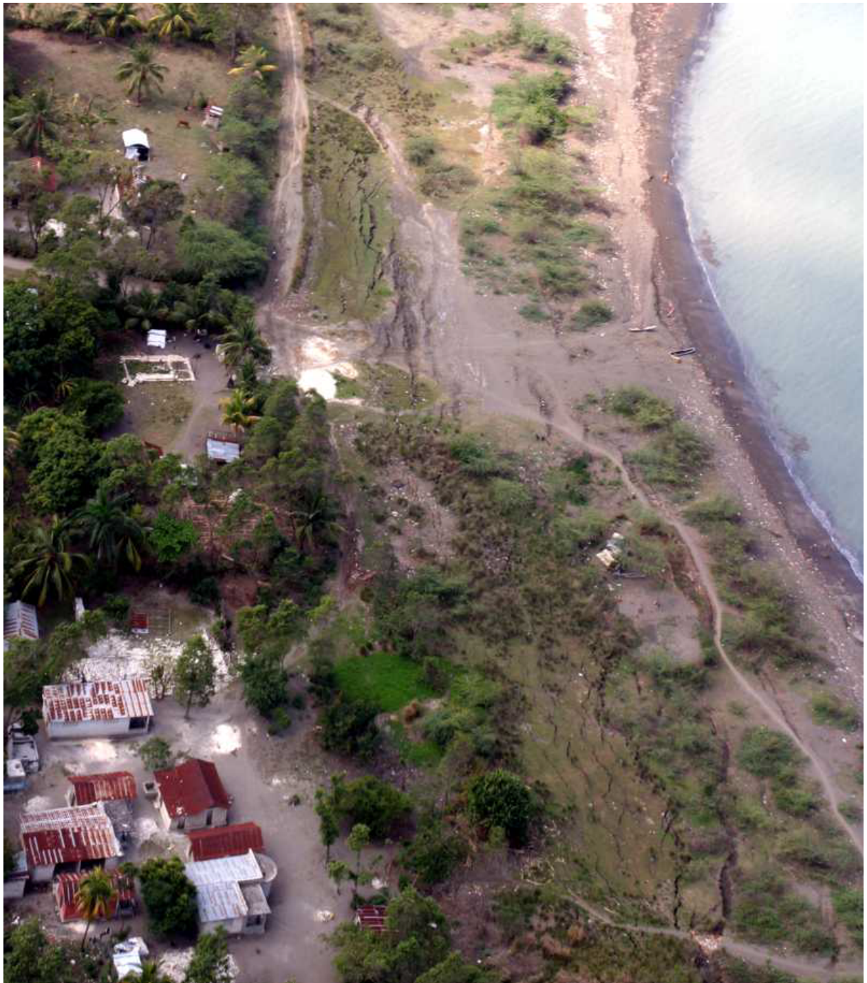
Figure 7. Lateral-spread cracks along coast west of Port-au-Prince near Léogâne.
