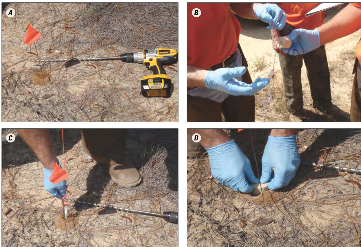
Figure 4. Installation of a passive soil-gas sampler includes (A) drilling a borehole in the soil with a stainless steel drill bit attached to a cordless drill, (B) attaching one end of a string to a sampler and the other end to a cork plug, (C) inserting the sampler on the string into the borehole, and (D) sealing the borehole with the cork plug to keep out surface contaminants.
