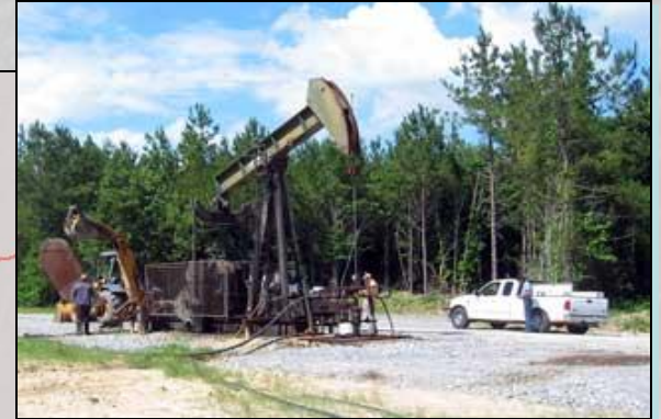
Service road paved with anhydrite
