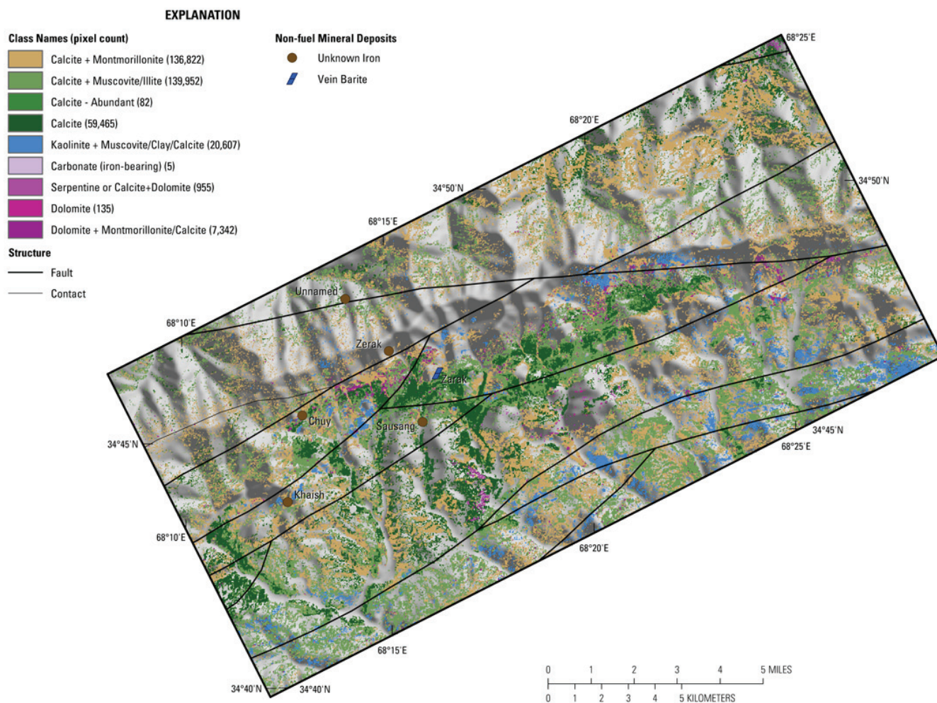
Figure 7B–30. Map showing the distribution of carbonate-bearing minerals in the Northeast Haji-Gak subarea detected in the HyMap data. The figure shows calcite, kaolinite, and dolomite within Paleozoic rocks in the southern half of the image.
