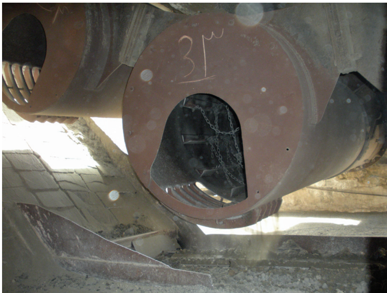
Figure 16B–14. Satellite cooler in operation at the Ghorl I cement plant. Photograph by Victor G. Mossotti, U.S. Geological Survey.
