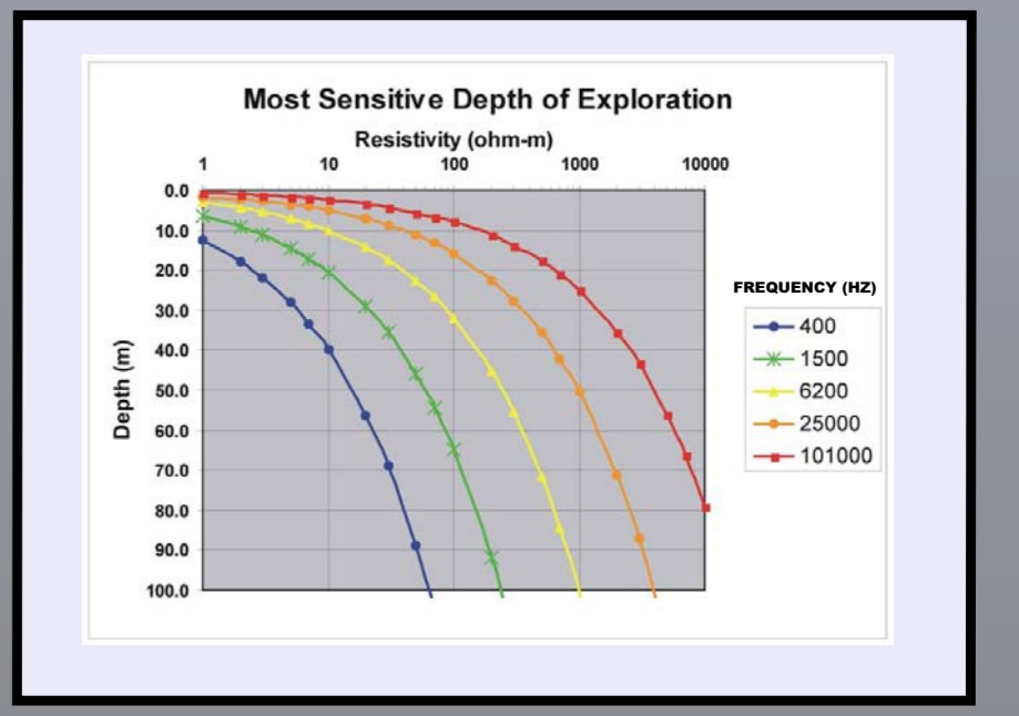
Each frequency penetrates to a different depth, depending on the bulk electrical resistivity of the earth. For high resistivity rocks, there is a good spread of penetration depths, making it possible to invert the data to obtain resistivity-depth profiles along the flight lines.
