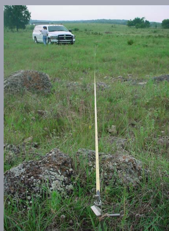
Stakes for electrodes are hammered into the ground at equal intervals along a straight ERI survey line.
