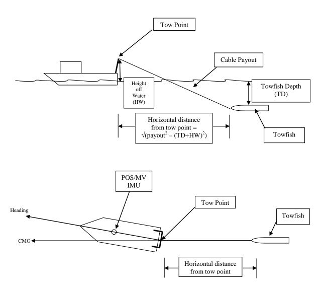
Figure A-6. Side Scan Towfish Position Calculations
